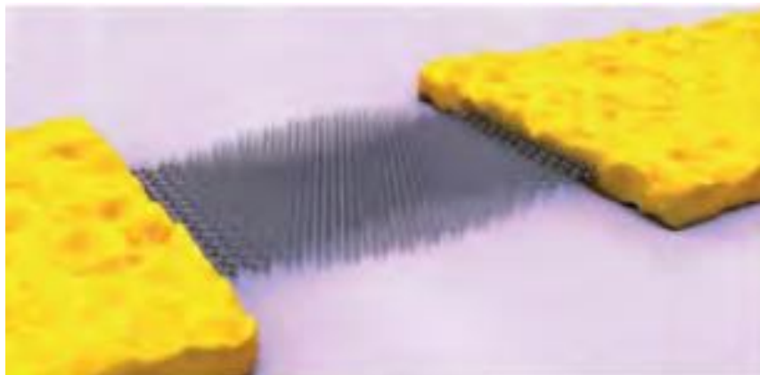
Fig 1.12 Nano-electromechanical sensor contains a graphene that connects to the two electrodes [13]
