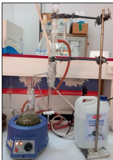
Figure 4: Extraction of essential oil by Hydro-distillation method.
