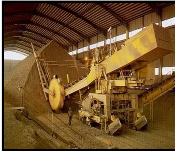
Figure.02: Raw prehomogenization hall [48].
