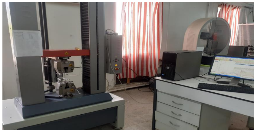
Figure III.5: Machine de traction (Zwick/Roell Z050) (Université Badji-Mokhtar Annaba).
