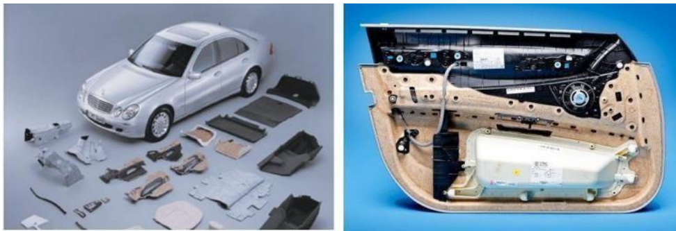
Fig. 1.12 Interior parts of vehicles of German manufacturers made of biocomposites [13]
