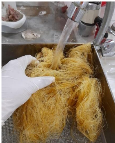
Fig. 2.15 Washing the fiber
