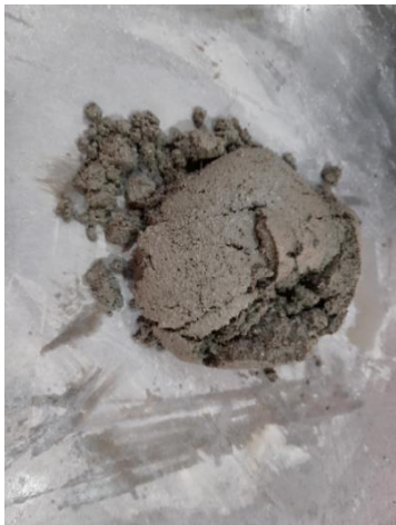
Fig. 2.24 Mortar after mixing
