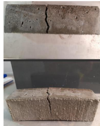
Fig. 2.37 Shape of mortar after bending test
