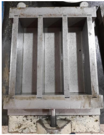
Fig.2.25 Steel prismatic mold of 40 \times 40 \times 160 \text{ mm}^2
