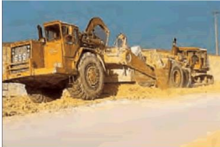
Figure II.2. Extraction en couche [5].
