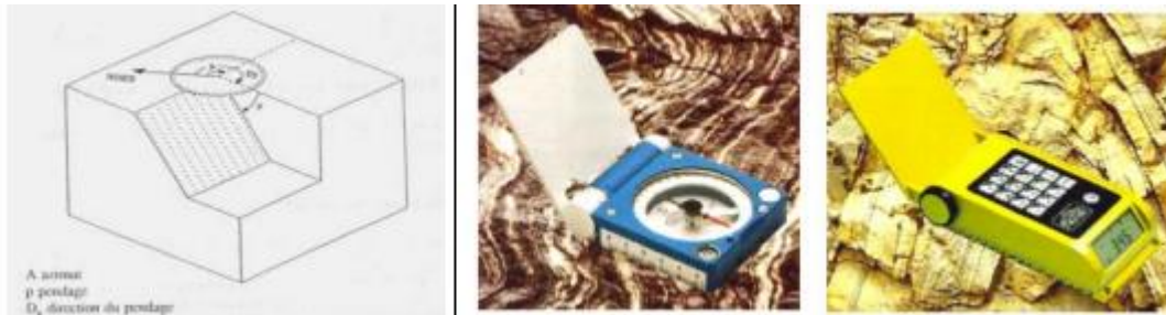
Figure I.10: Orientation of a discontinuity and measuring equipment. [1]
