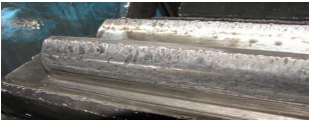
Figure I.10 : Grippage des dents.
