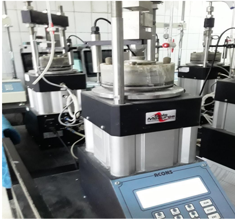
Figure 44: Set the loading frame with a loading platform.
