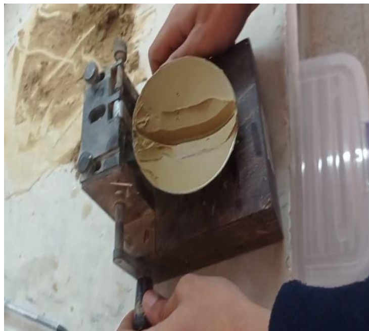
Figure 38: Grooving the Portion in the cup of the Casagrande.
