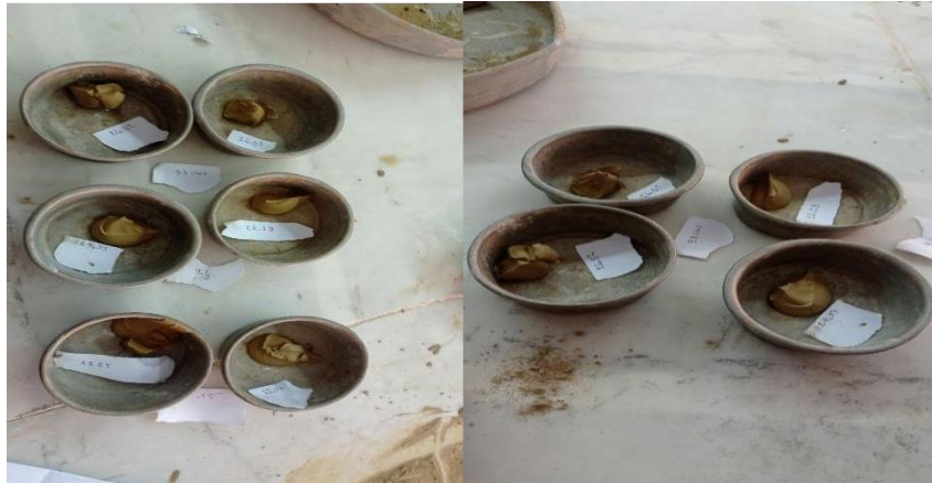
Figure 39: Determination of moisture content
