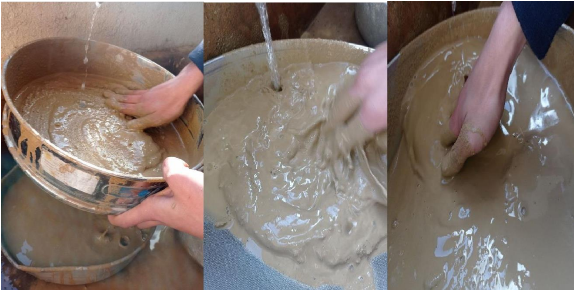
Figure 36: Washing the samples through a 0.4mm sieve.
