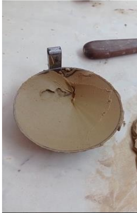
Figure 37: portion of the moist soil sample in the cup of the Casagrande.
