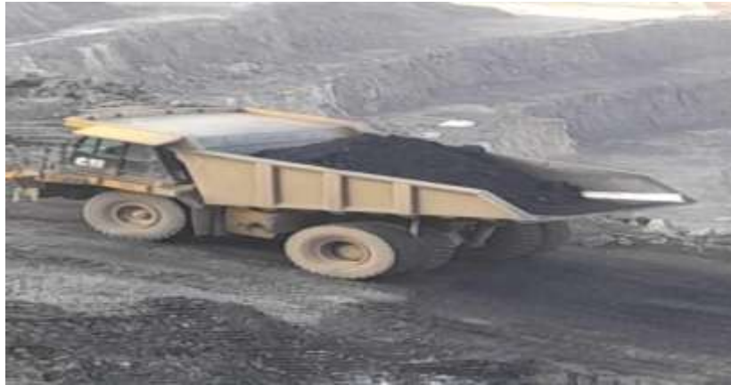
Figure II.6: camion CATERPILLAR de type 775G
