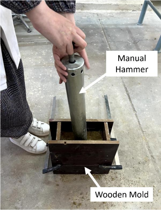
Figure 5.8 The adopted rammed earth compaction process
