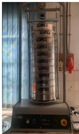
Figure 4.1 The sieving machine used for the sieve analysis
