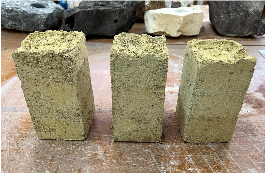
Figure 5.5 10x10x20cm prismatic specimens with Lime Stabilization
