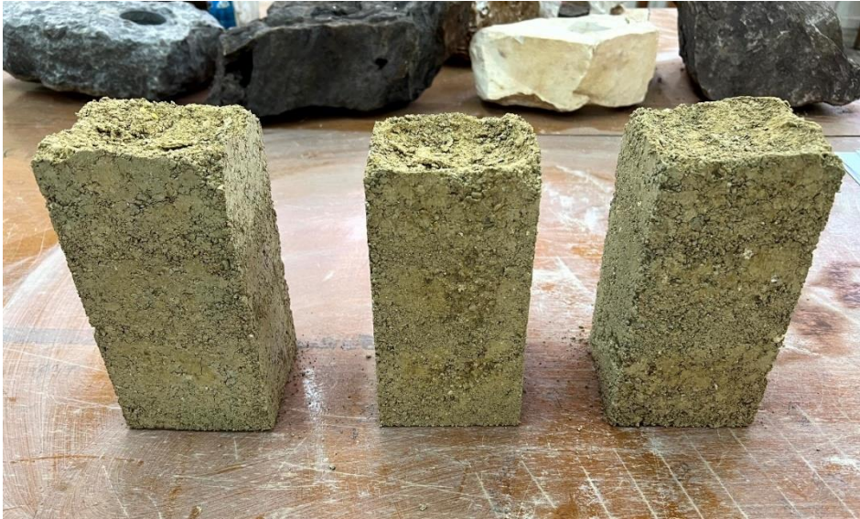
Figure 5.6 10x10x20cm prismatic specimens with Cement Stabilization
