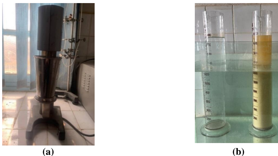
Figure 4.3 Earth material dispersion mixer (a) and the prepared two graduated glass cylinders (b)
