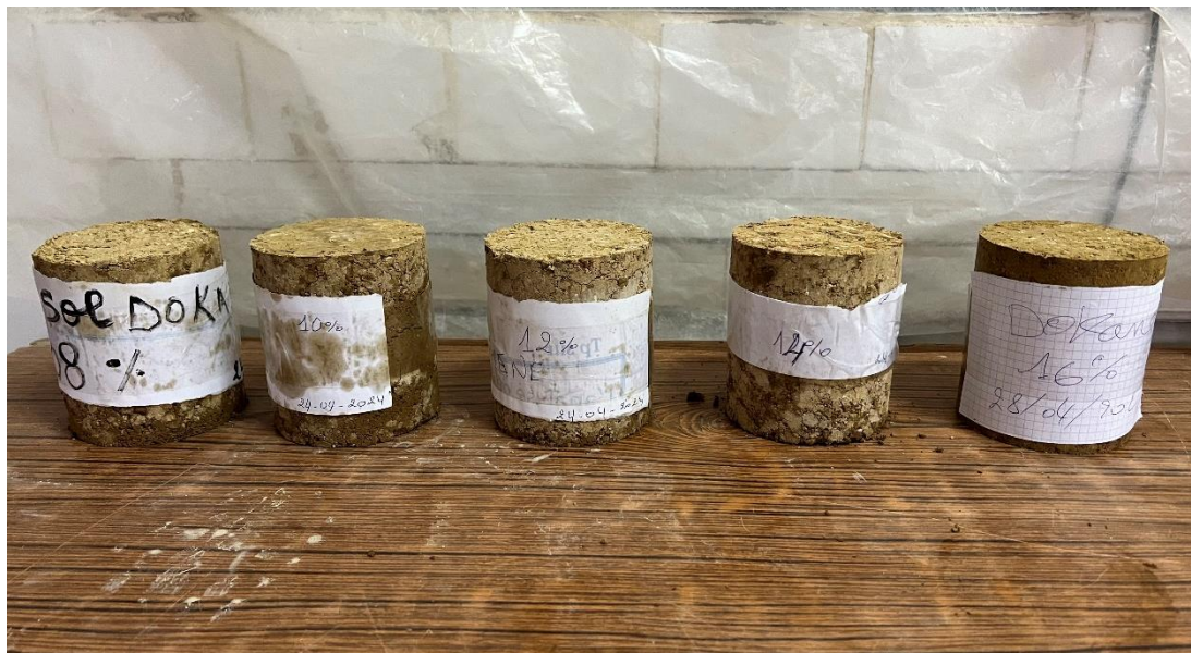
Figure 4.7 Standard Proctor cylindrical specimens after compaction
