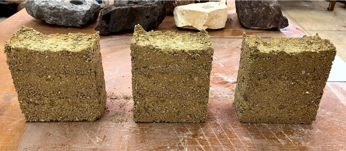
Figure 5.10 10x20x20cm prismatic specimens without Fiber reinforcement
