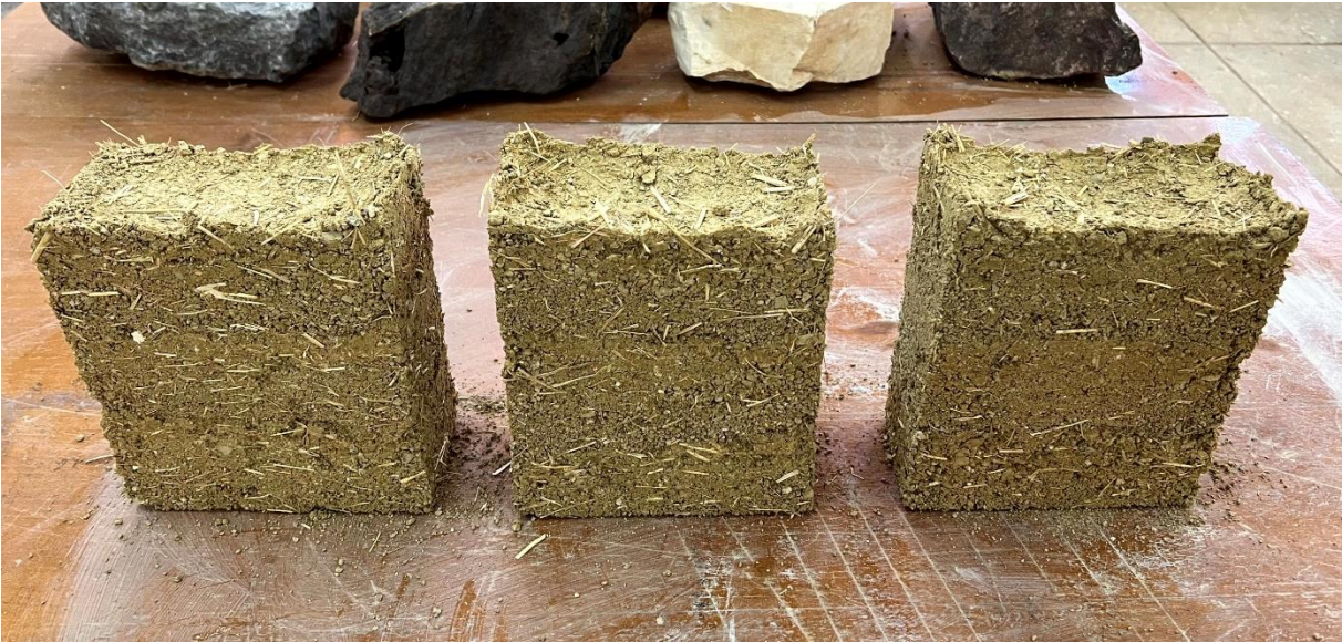
Figure 5.11 10x20x20cm prismatic specimens without Straw Fiber reinforcement
