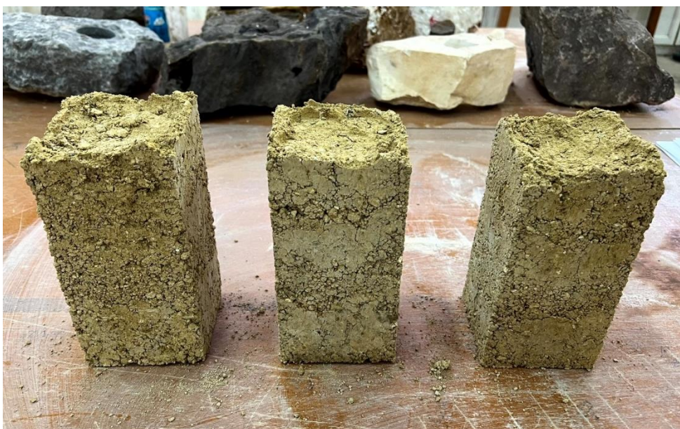
Figure 5.3 10x10x20cm prismatic specimens without Stabilization
