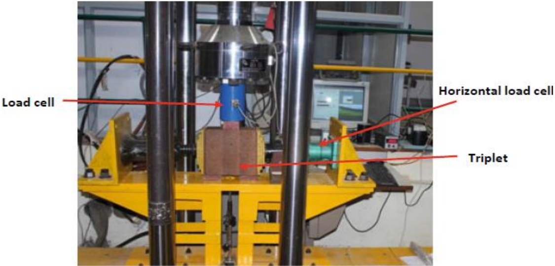
Figure 3.8 Triplet shear test set-up (Venkatarama reddy, 2022)
