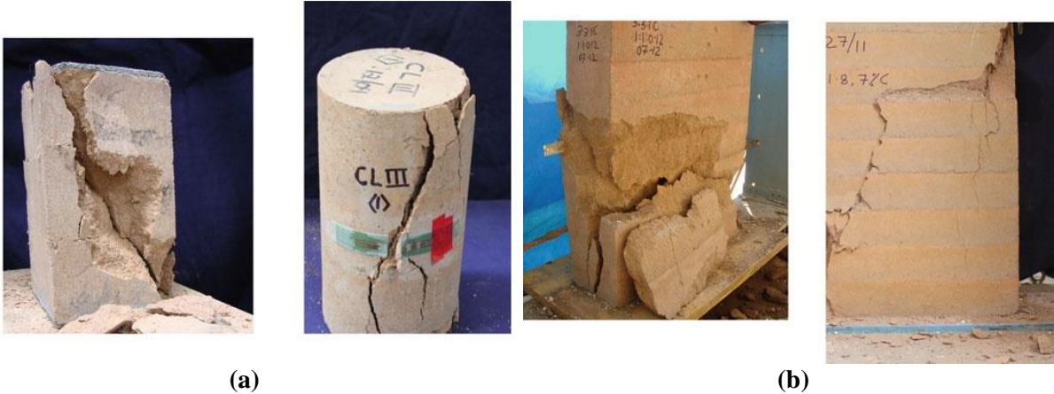
Figure 3.7 Failure patterns for RE prism, (a) Cylinder and (b) Walette specimen (Venkatarama reddy, 2022)
