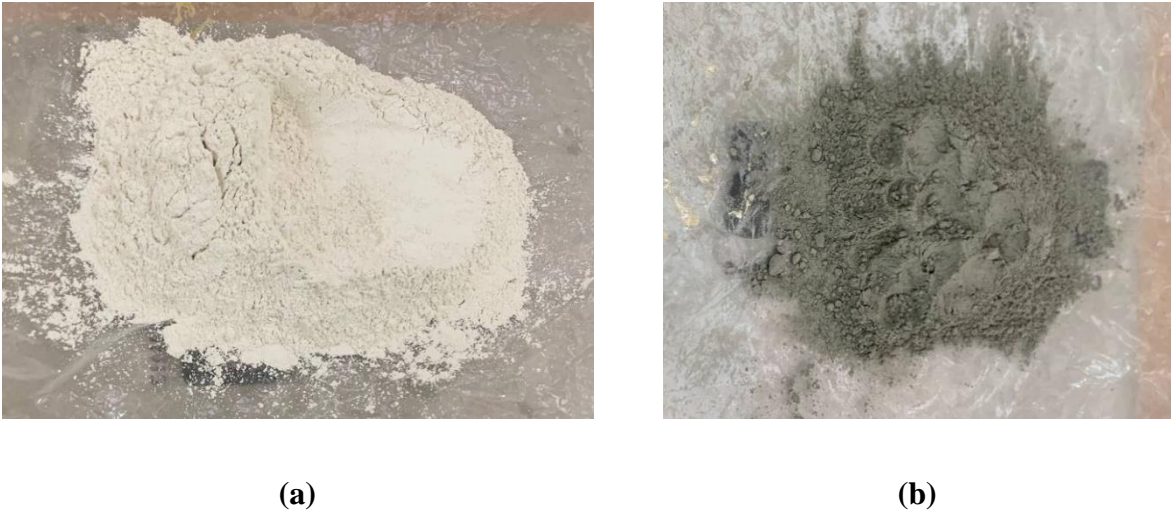
Figure 5.4 The stabilization material used: Lime (a) and Cement (b)
