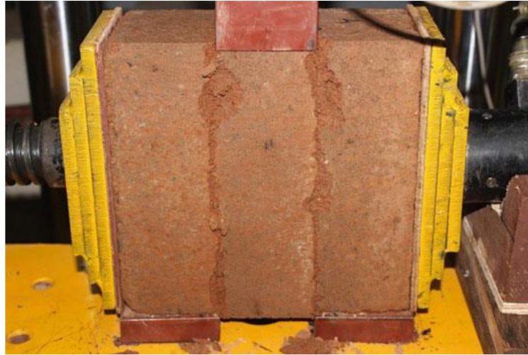
Figure 3.9 Failure along the interfaces of triplet specimen (Venkatarama reddy, 2022)
