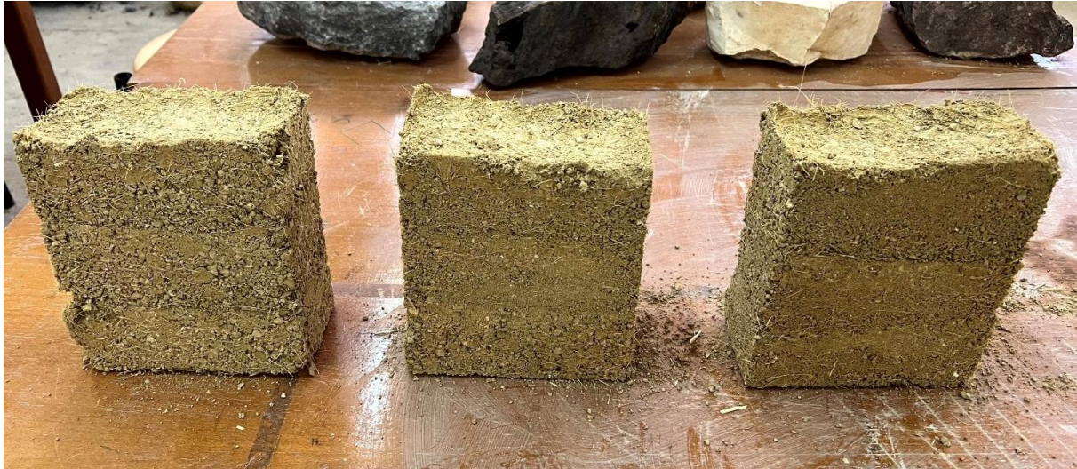
Figure 5.12 10x20x20cm prismatic specimens without Coir Fiber reinforcement
