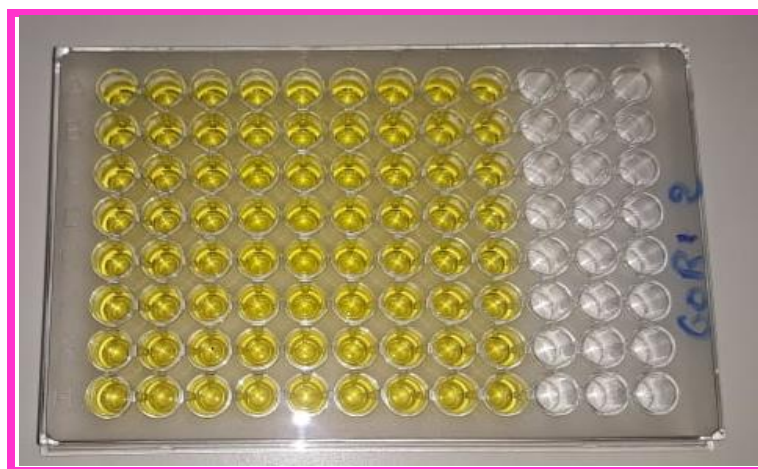
Figure 35: Galvinoxyl assay (GOR) results on the microplate.
