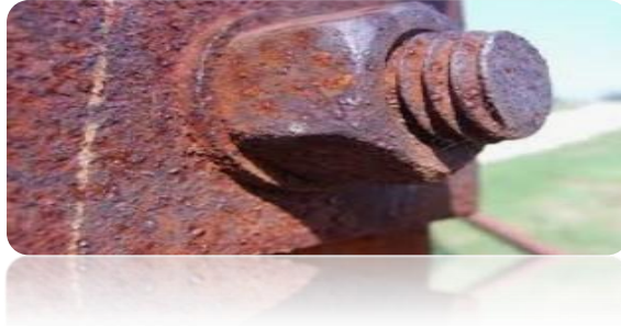
Figure I.4: La corrosion galvanique
