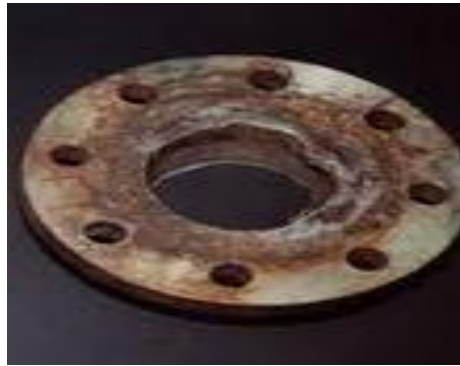
Figure I.5: La corrosion caverneuse
