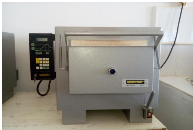
Figure II.6: Four de la marque NABERTHERM.
