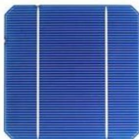
Figure I.5—Cellule monocristalline. [1]
