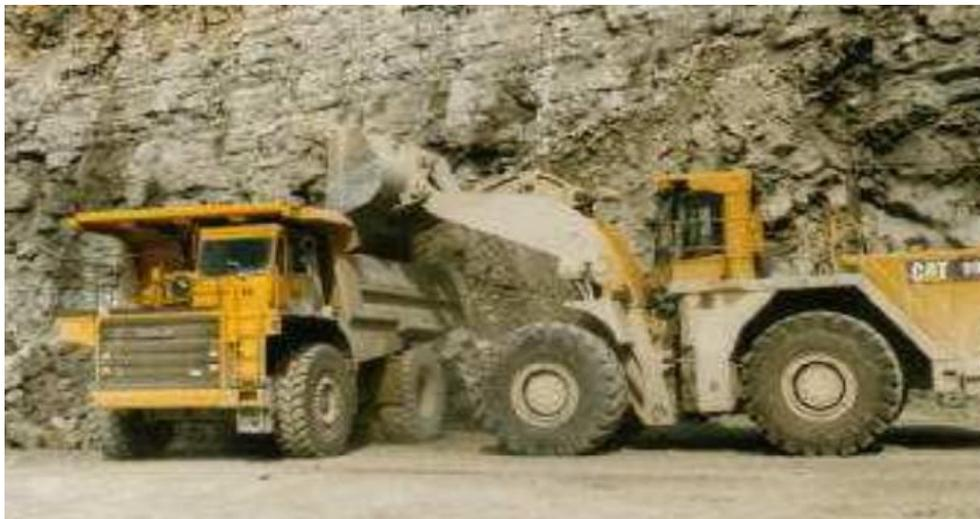
**Fig.2.6.** Chargement des engins de transport [19]
