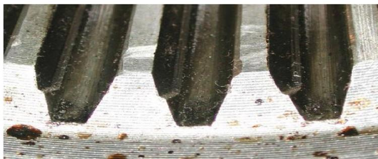
Figure I.14:Usure abrasive "Engrenages"[13].
