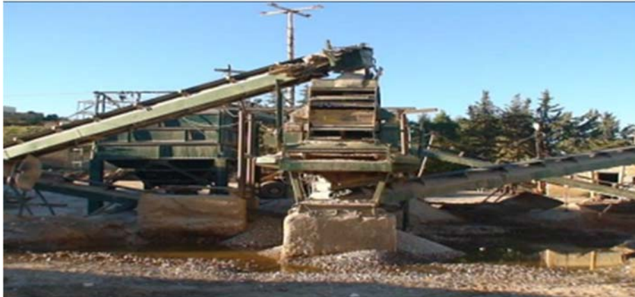
Figure III.3 : Crible vibrant de Ain Mimoun.
