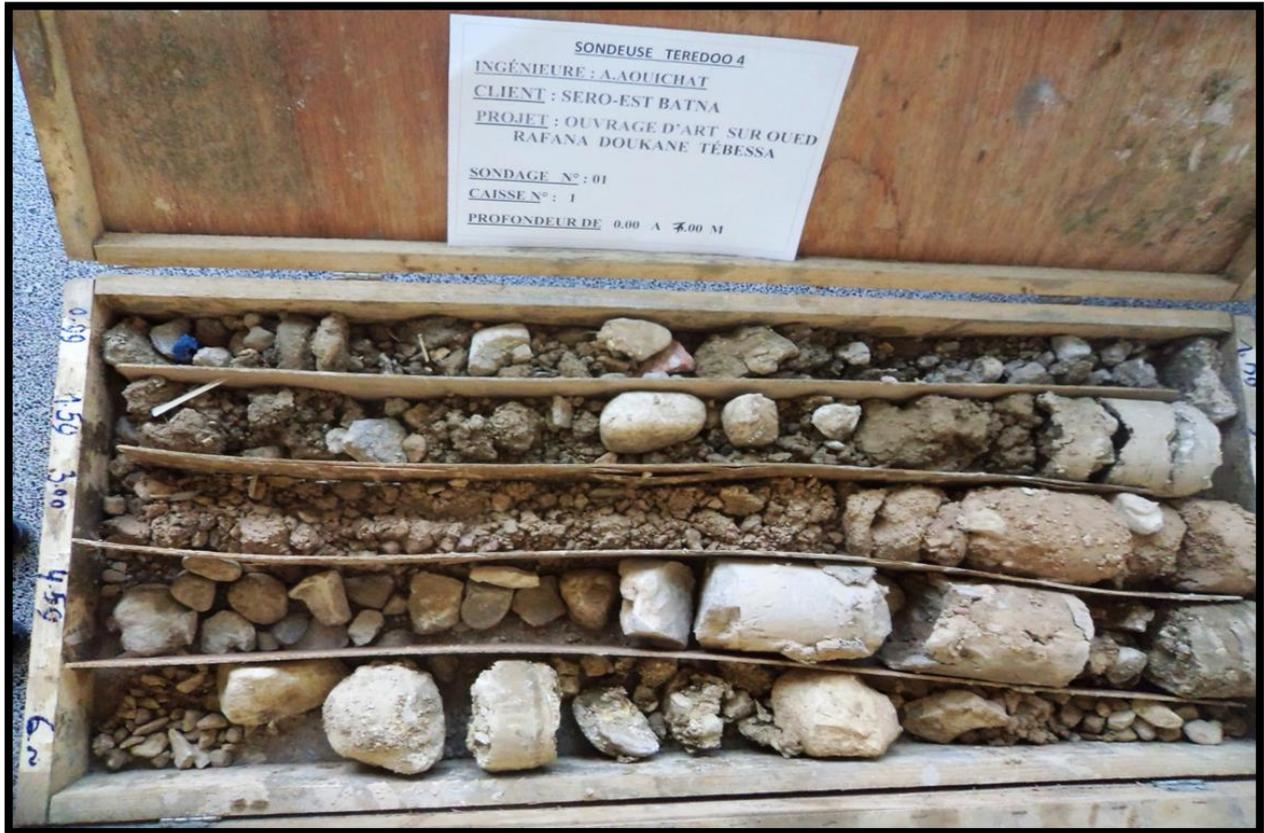
FIGURE 9: SONDAGE 01 CAISSE 01 PROFONDEUR 0.00-7.00 M OUVRAGE D'ART RAFANA
