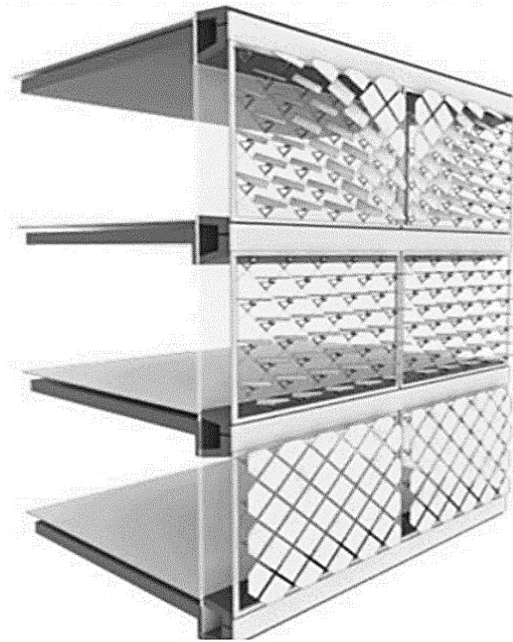
Figure 16: la façade adaptive solaire a cellules photovoltaïques
