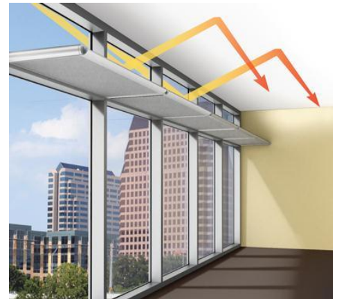
Figure 1-5. un light shelf. Source: Designing Buildings Ltd, 2021
