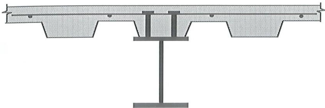
Figure 1.11 Composite Beam with Ribbed Metal Deck
