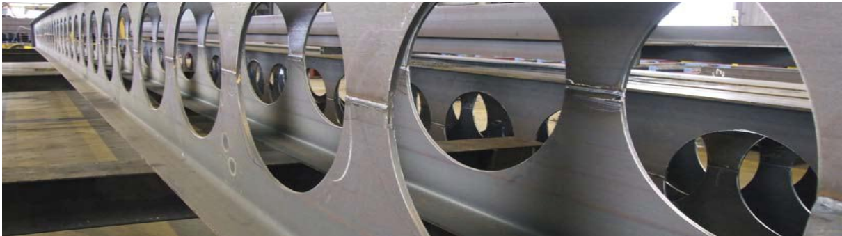
Figure 1.4: Example of cellular beams
