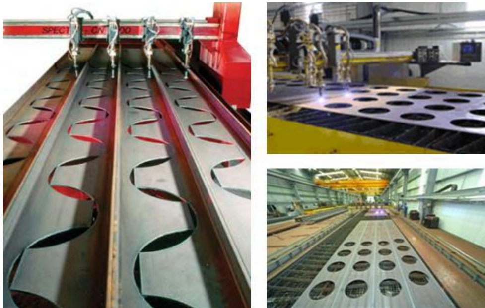
Figure 1.12: fabrication process of perforated steel beams.
