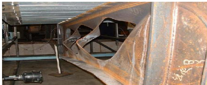
Figure 2.4: Lateral-torsional buckling due to (vertical) shear.
