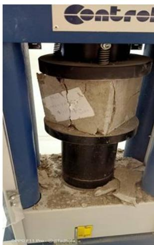
Photo 4.1: Machine de compression
