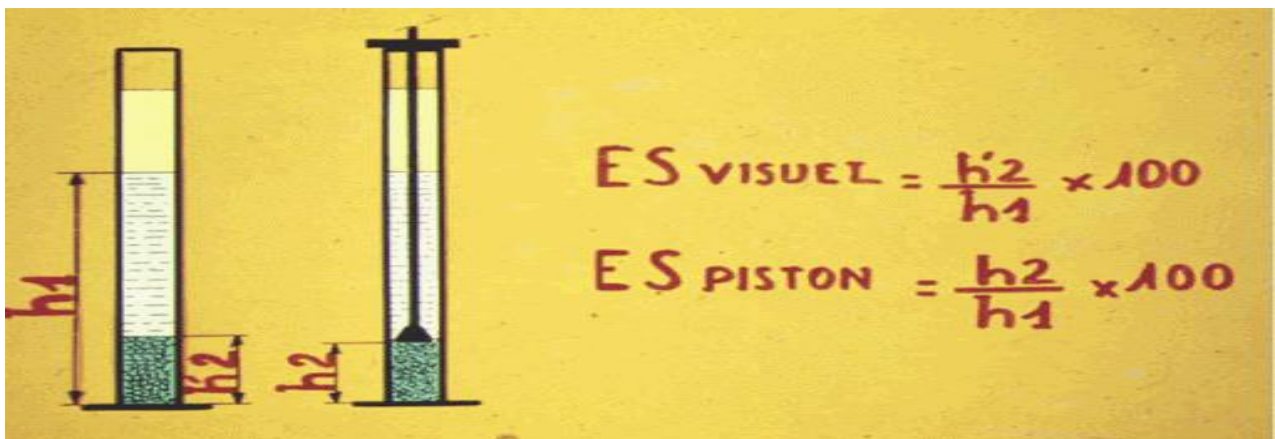
Figure III. 4. essai Equivalent de sable
