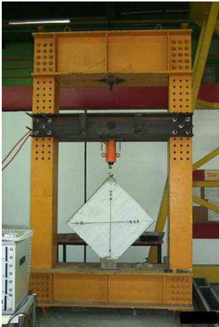
Figure 2.16 : Essai RILEM de compression diagonale. [1]
