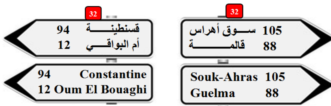
Figure 11.9 Signalisation de direction type E [15].
