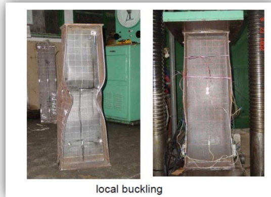
Figure 1.2 Experimental local buckling in flanges and web of steel member
