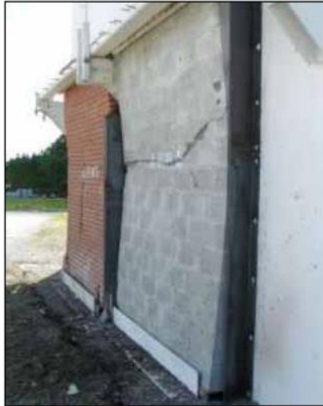
Figure 3-6 Result of Full-Scale Explosion Testing of Fully Grouted CMU and Cavity walls [27]
