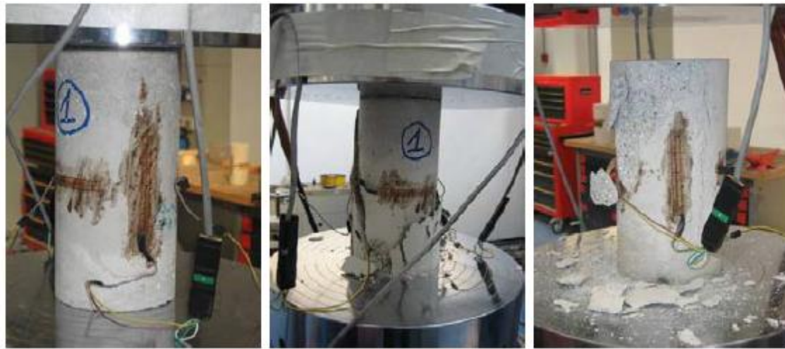
Figure 5-6 Compression test on mortar cylinder
