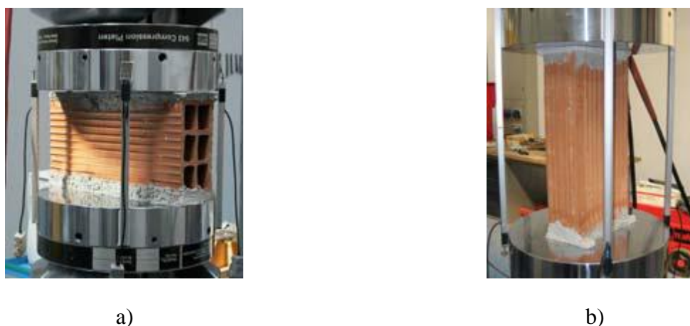
Figure 5-1 hollow brick compression tests: a) compression orthogonal to holes, b) compression parallel to holes
