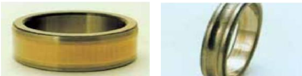
Figure IV.11 : Corrosion de contact.
