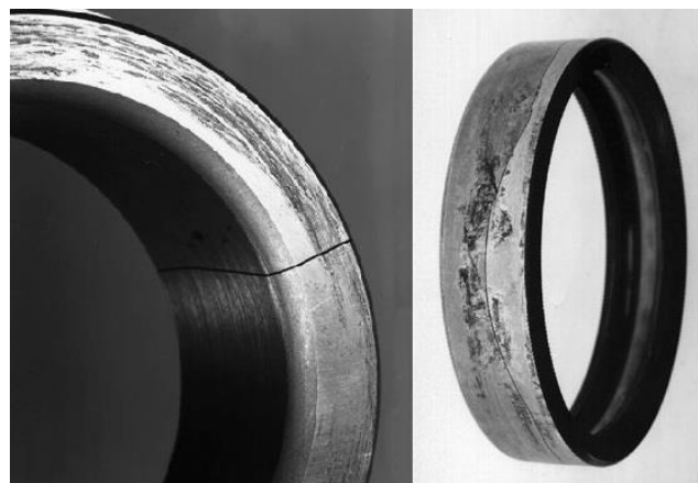
Figure III-7: Exemples de fissure
