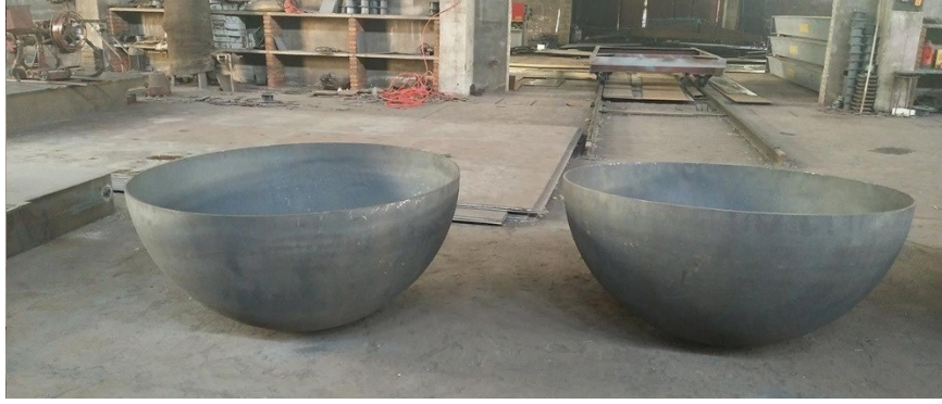
Figure 2.20 Hemispheric bottom of the tank
