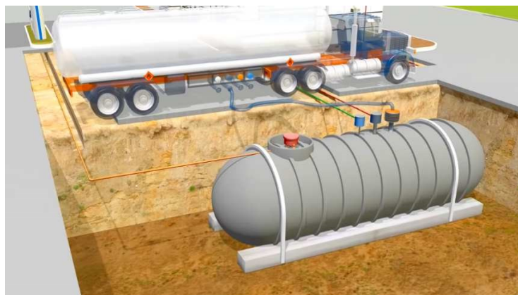
Figure 1.3.2 underground Storage tanks
