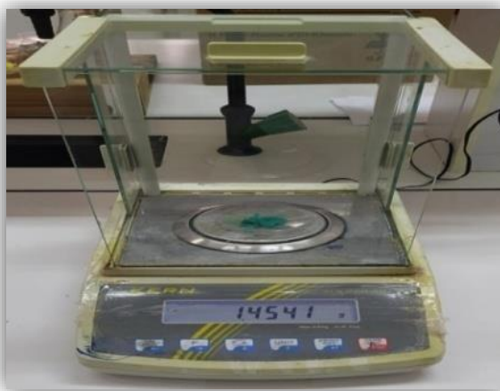
Figure III.1: Sensitive electronic balance at four digits ( 10^4 g) sensitivity.
