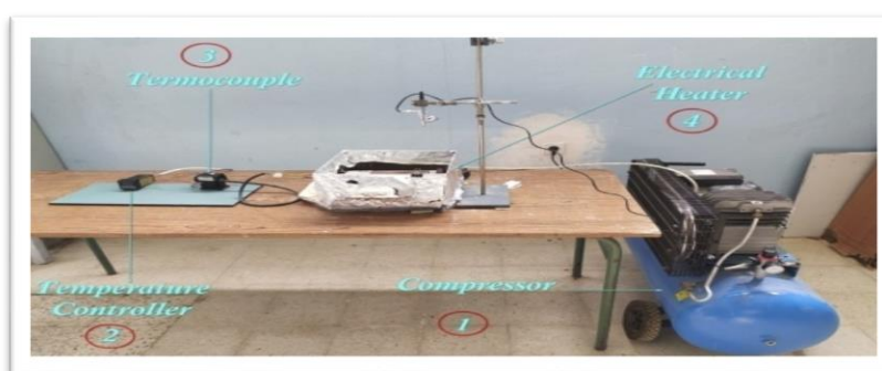
Figure III.8: Experimental setups of the homemade pyrolysis spray system.
