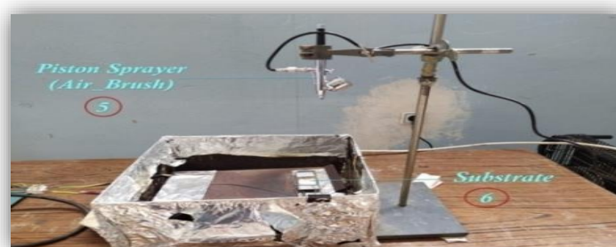
Figure III.9: Experimental homemade device of the pyrolysis spray technique.
