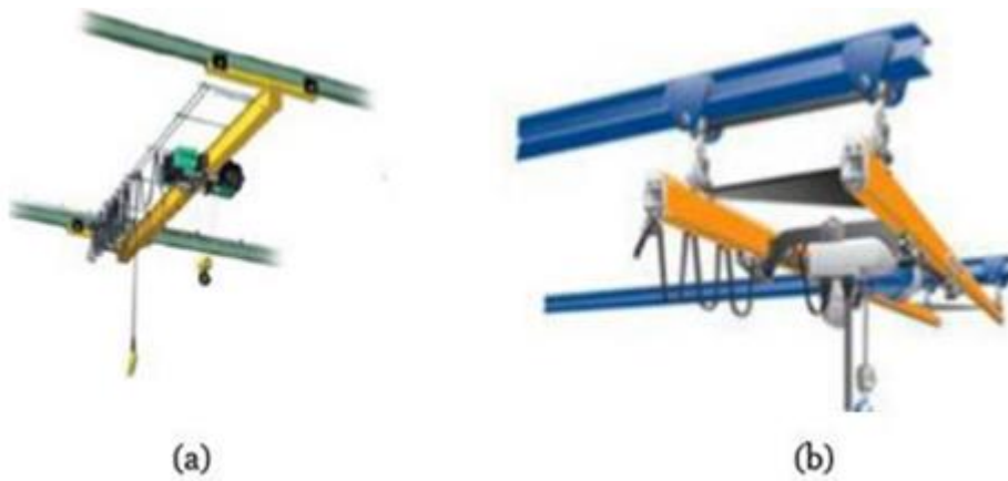
Figure I.5 (a) mono poutre suspendu (b), bipoutres suspendu
