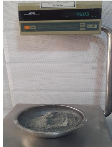
c. measuring the cement
