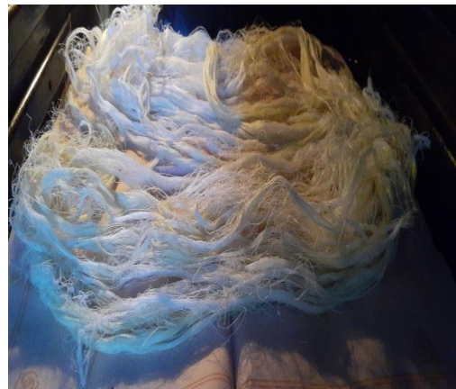
Fig 3.16 The treated fibers drying in the oven.
