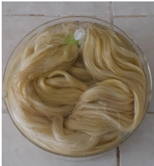
Fig 3.14 The fibers soaking in 2% sulfuric acid somution for 10 min.
