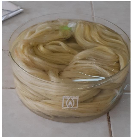
Fig 3.14 The fibers soaking in 2% sulfuric acid somution for 10 min.
