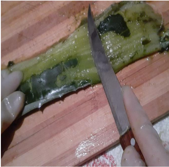
Fig. 3.4 Crushing of Agave Americana fibres
