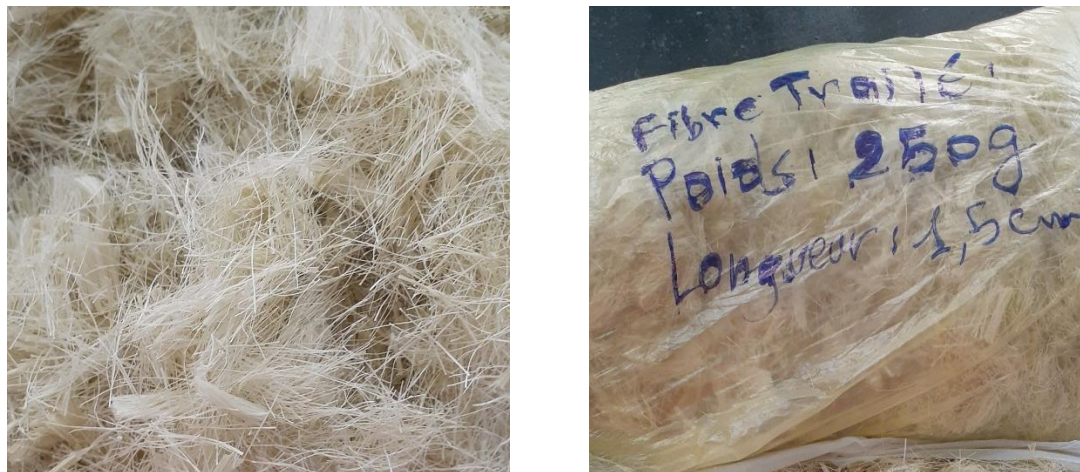
a. Fibers cut to 15 mm length
