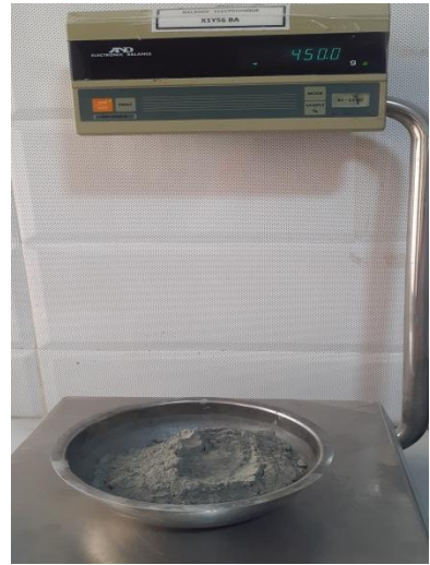
c. measuring the cement
