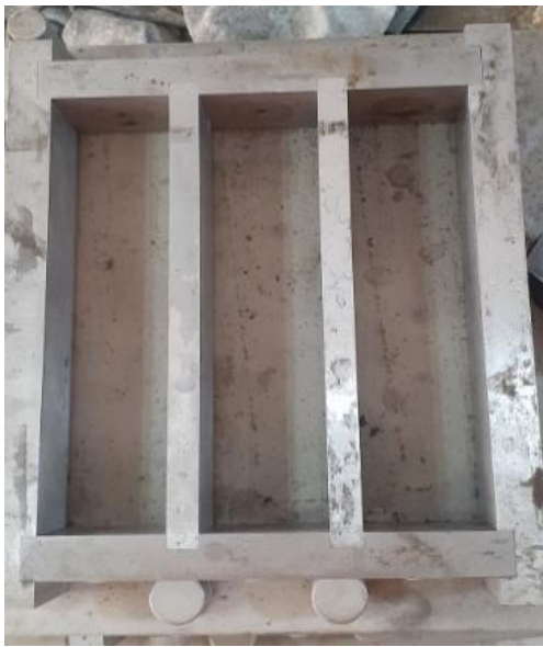
Fig 3.21 Steel prismatic mold of 40×40×160 mm 3
