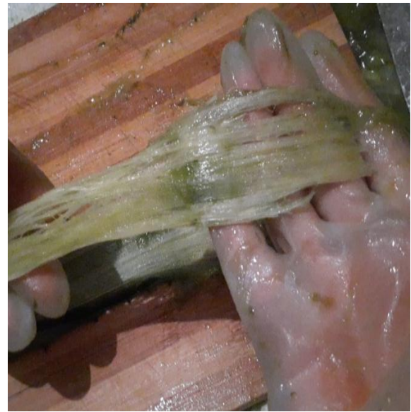
Fig. 3.5 Extraction of Agave Americana fibers
