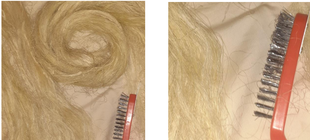
Fig 3.17 Brushing of treated Agave Americana fibers
