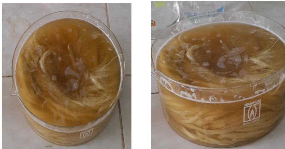
Fig 3.11 The fibers after soaking for 4 hours in NaOH solution.
