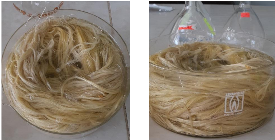
Fig 3.10 The fibers soaked in 2 % Soda Solution.
