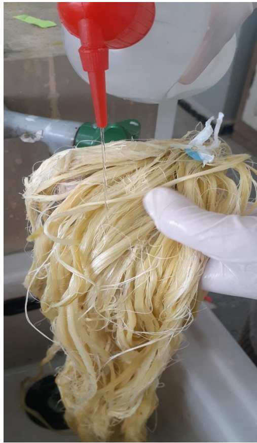
b. washing the fibers with distilled water for 15 minutes until neutral pH
