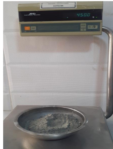
c. measuring the cement
