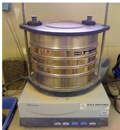
FIGURE IV.2 : TAMISEUSE A VIBRATIONS
