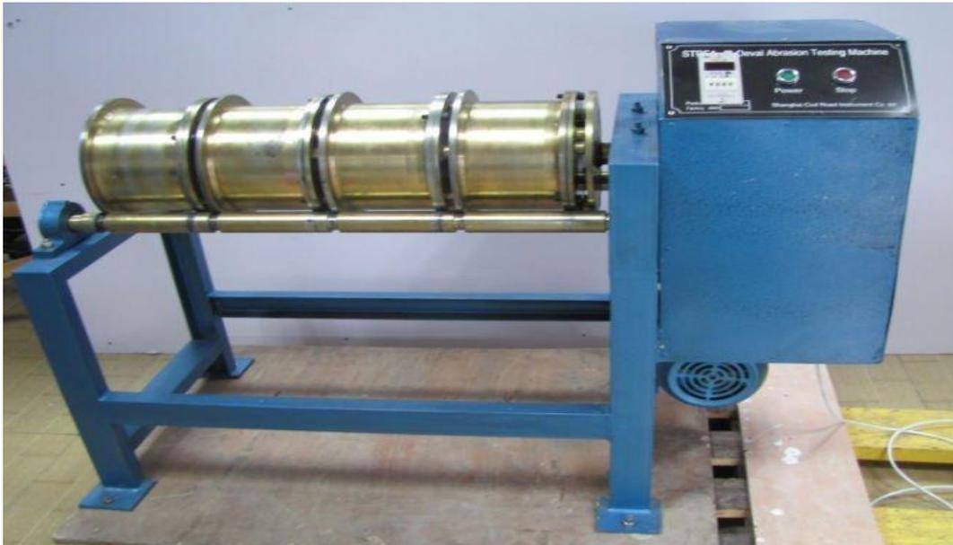
**FIGURE IV.9: L'ESSAI MICRO DEVAL**
