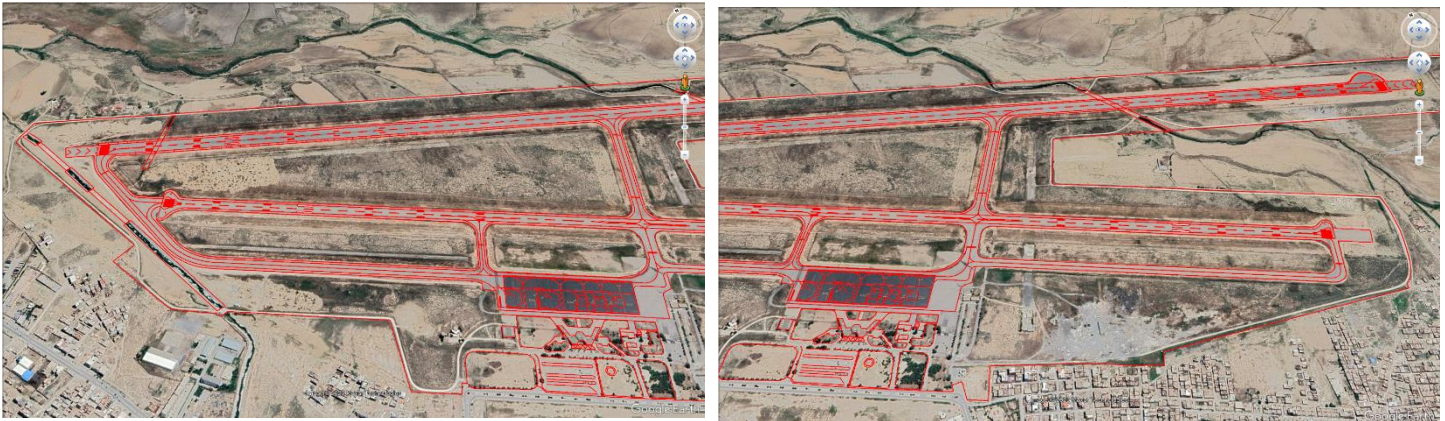
Fig 5.1 Two screenshots showing how to draw an aerodrome using Google Earth Pro.
