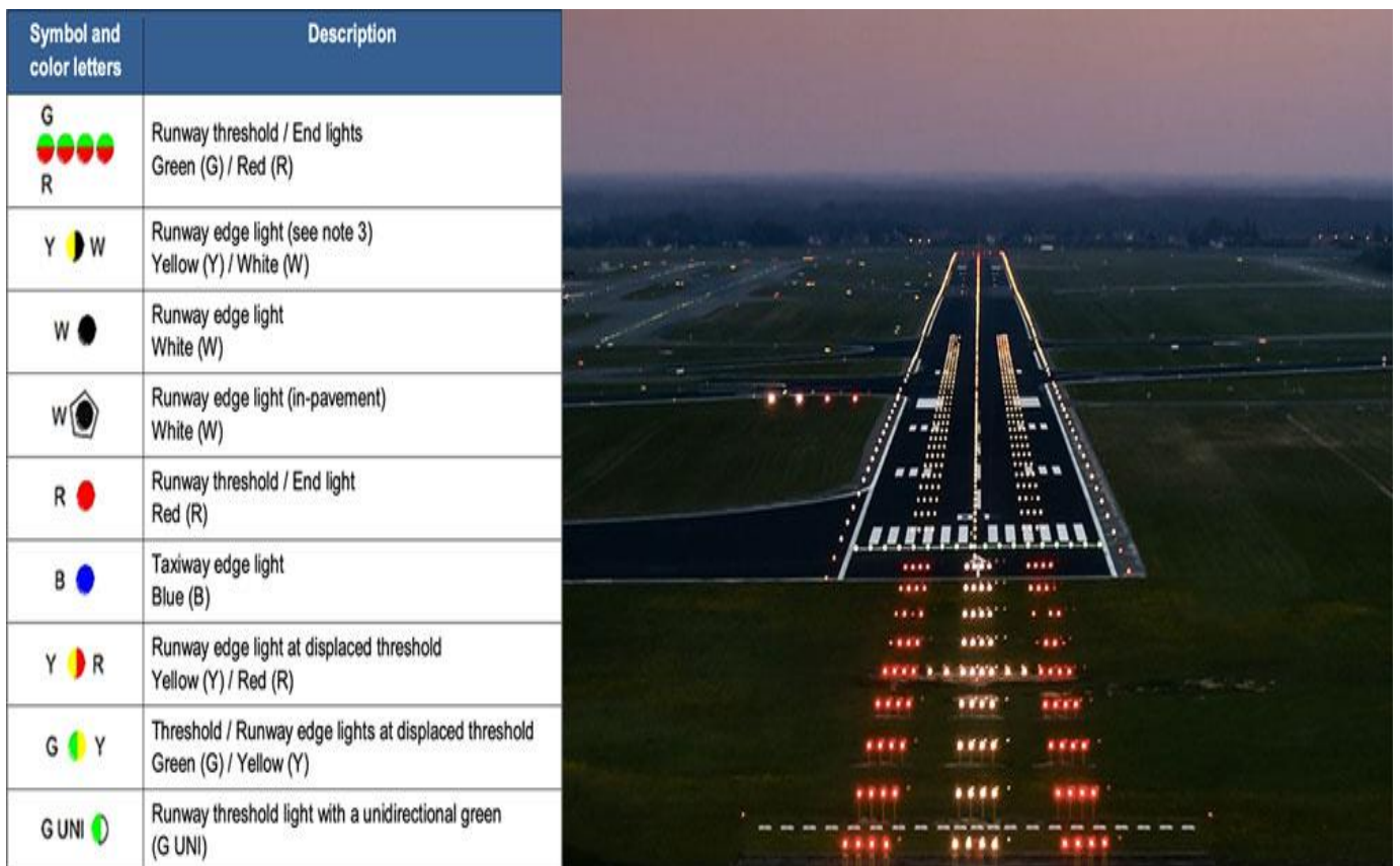
Fig 4.11 Colors Found In Runway Edge Lighting. [31]
