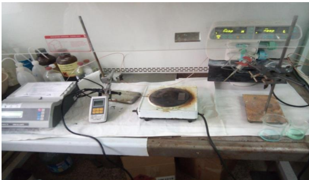
Figure II.3. Equipment used in ultrasonic spray pyrolysis technique.
