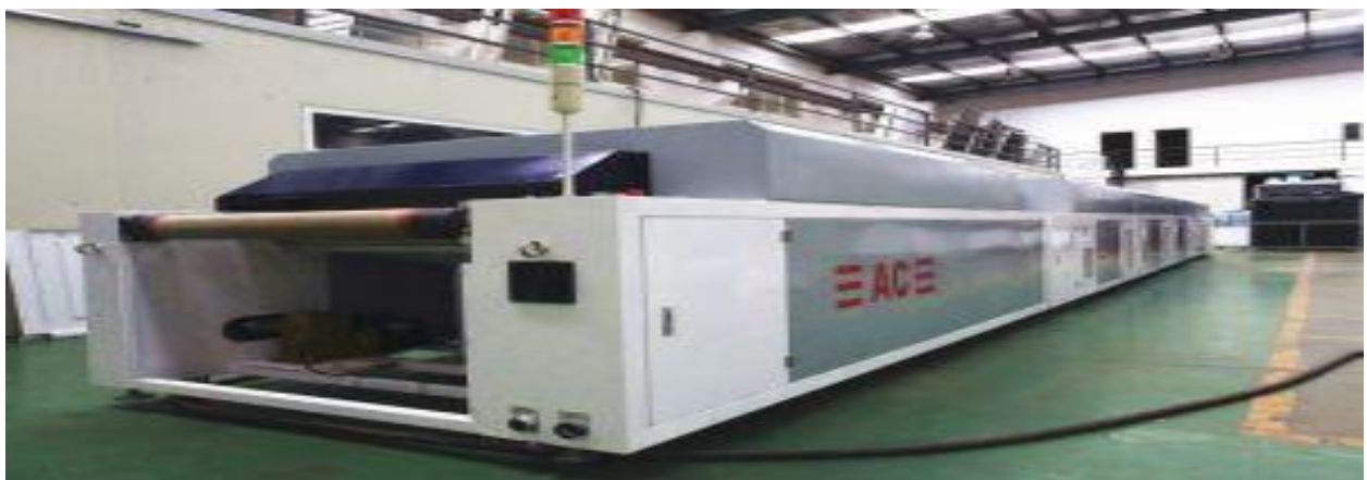
Figure II.10 : Tunnel de séchage [11]
