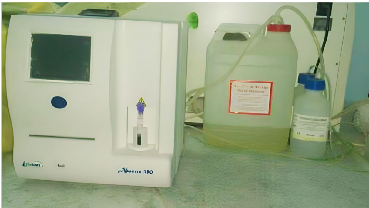
Figure 14: Abacus 380 biochemical automaton with 19 parameters
