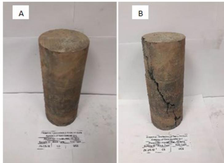
Fig 27: Uniaxial Compressive Strength Sample ZK03
