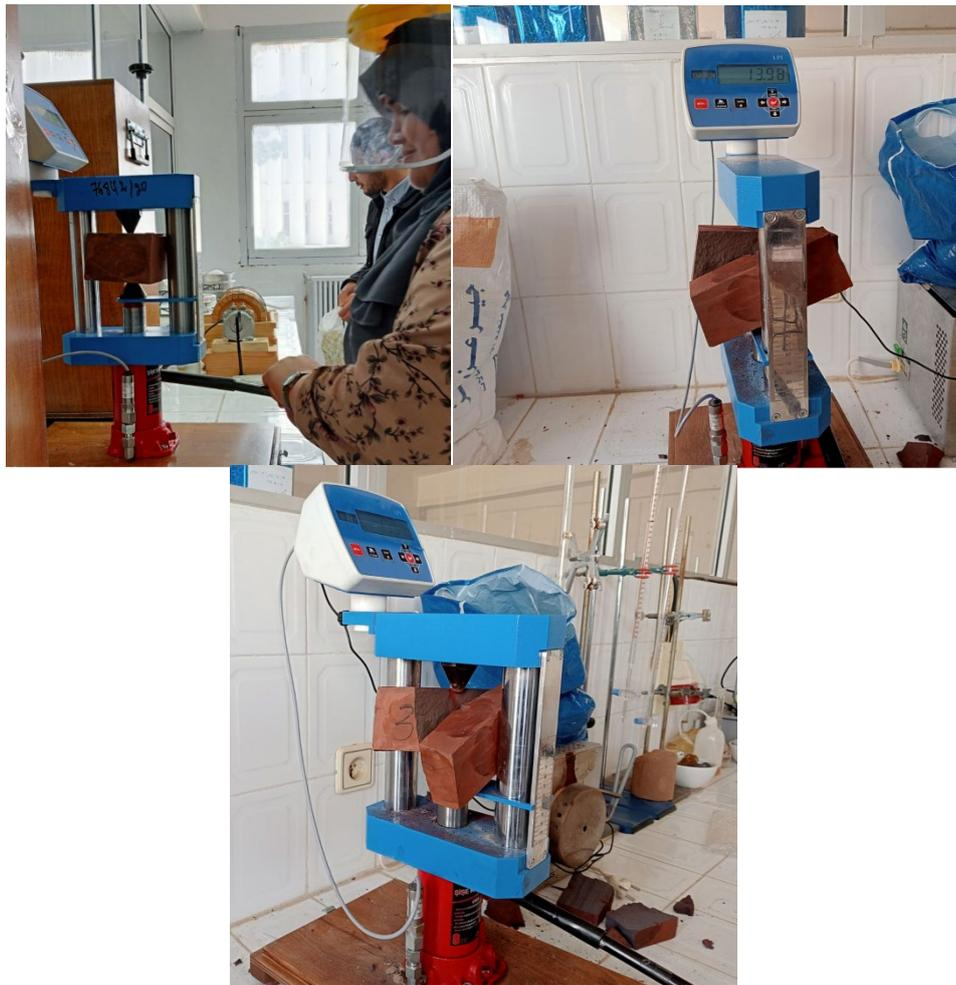
Fig 30: Photos of realization test point load
