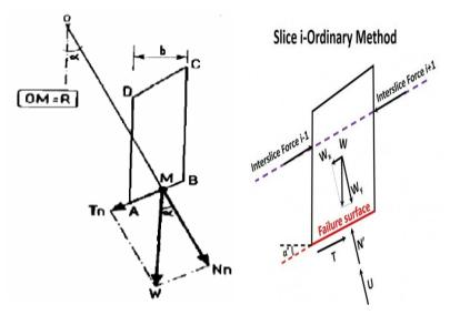
Fig 34: Forces acting on a surface according to FELLENIUS. [53]
