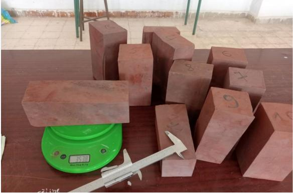
Fig 28: Photo of realization the density of ironstone Table III-7: Value density of ironstone
