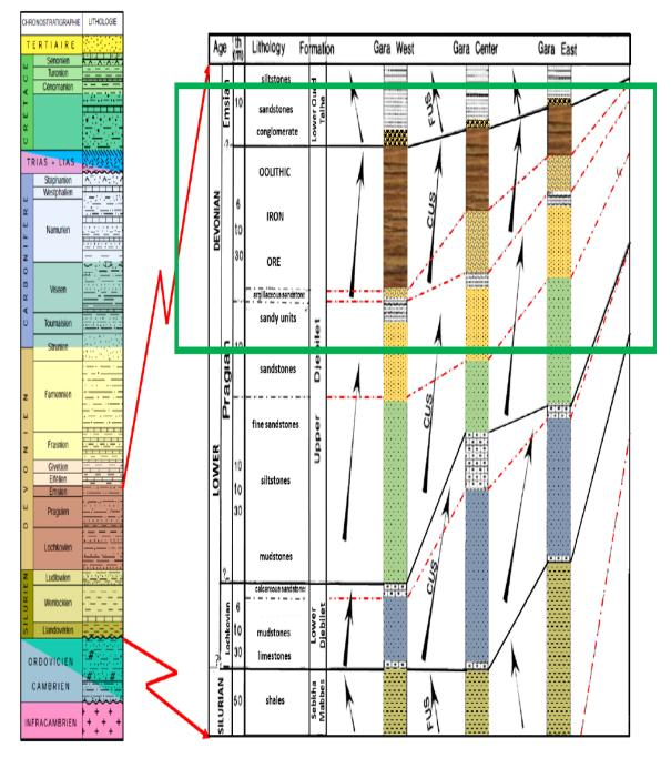
Fig 15: Lithostratigraphic columns of the Gara Djebilet deposit. [30]
