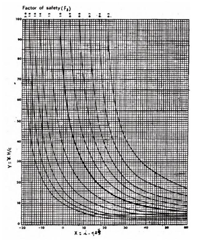
Fig 38: Hoek chart for calculating the safety factor (Fs). [71]
