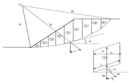
Fig 32: Description of slicing with breaking surface. [54]
