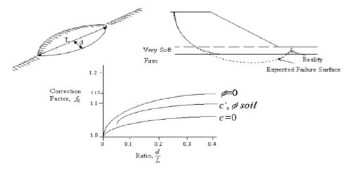
Fig 36: Variation of the correction factor according to depth and length of the fracture surface. [61]
