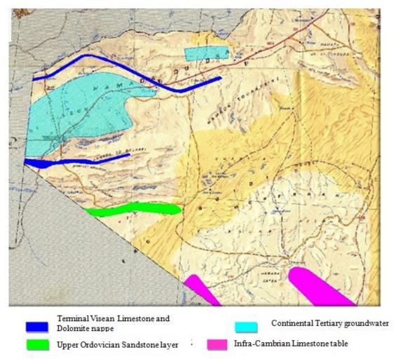
Fig 9: Schematic map showing the distribution of the different aquifers of the Tindouf basin [23]
