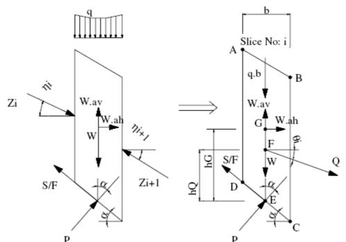
P Fig 37: Representation of forces on a slice using the simplified method of Morgenstern and Price. [72]
