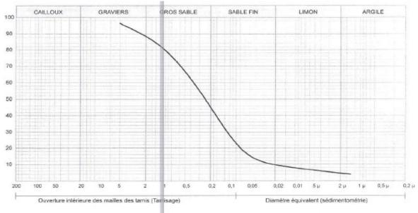
Fig 21: Particle size curve ZK08/0.2-0.7 (Fine-grained sandstone)
