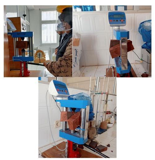
Fig 30: Photos of realization test point load Table III-9: Value de PLT and resistance of compression under point load
