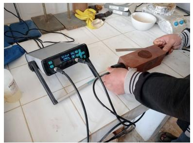
Fig 38: Photos of realization ultrasonic test of ironstone
