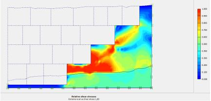
Fig 46 : Relative shear stresses
