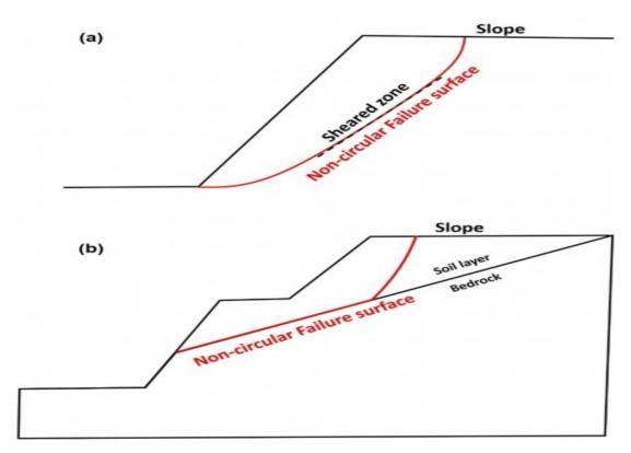
Fig 31: Description of the failure surface. [54]
