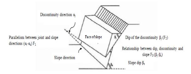
Fig 20: Orientation of a flat slope. [42; 43; 44;51]
