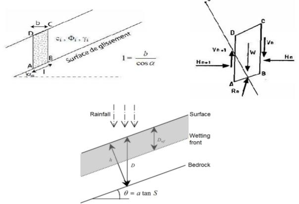
Fig 33: Demonstration of forces acting on a wafer. [54]
