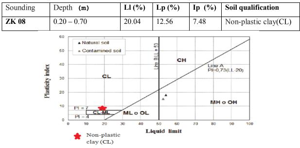
Fig 22: Curve of Atterberg limits ZK08/0.2-0.7
