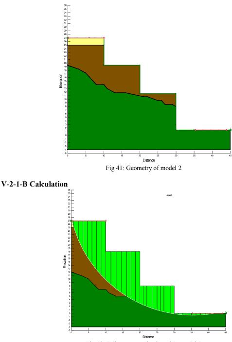
Fig 42: Failure area and value of Fs model 1
