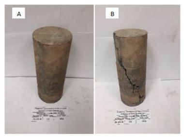
Fig 27: Uniaxial Compressive Strength Sample ZK03 A (Before) B (After)
