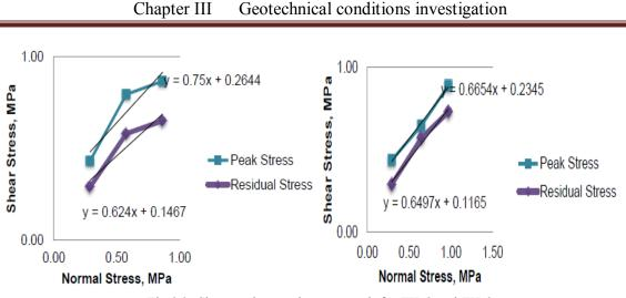
Fig 26: Shear and normal stress graph for ZK-8 and ZK-3
