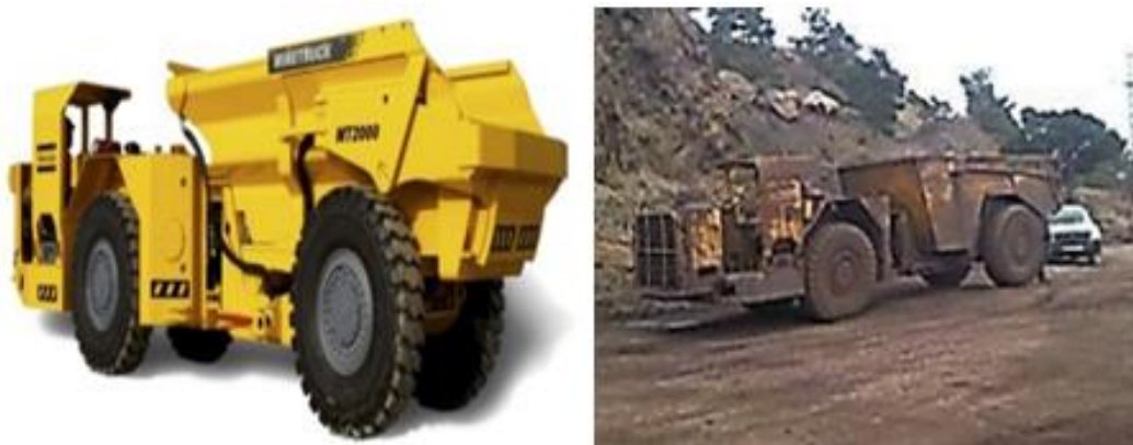
Figure II.13. Camion navette ATLAS COPCO MT2000.
