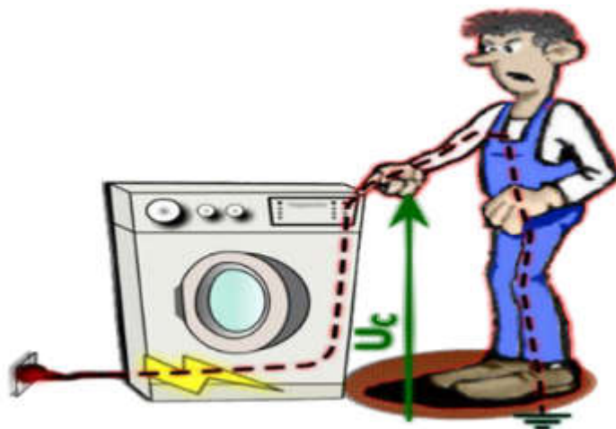
Figure 2.11 Tension de contact
