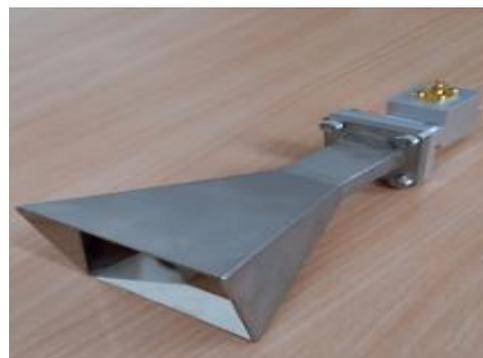
**Figure I.5 :** Antenne cornet.
