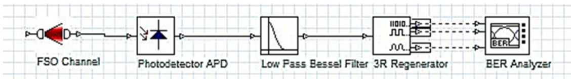
Figure 1.17: FSO receiver using APD photodetector.
