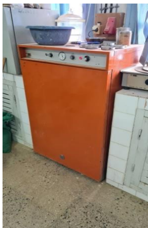
Figure 23: Etuve réglable (50°C-105°C)
