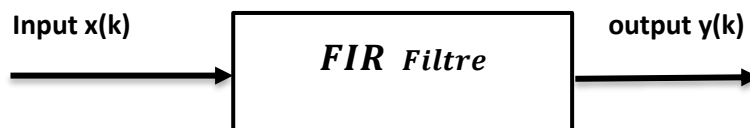
Figure 1.9: non-recursive discrete FIR Filter
