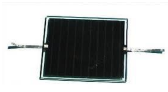
Figure II.7 High efficiency multi-junction solar cell
